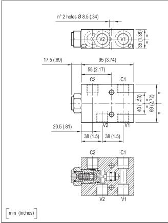
Flow is allowed to pass from V2 to C2 when pressure at V2 rises above the spring bias pressure and the poppet is pushed from its seat. The valve is normally closed (checked) from C2 to V2; when sufficient pilot pressure is present at V1-C1 the pilot piston acts to push the poppet from its seat and flow is allowed from C2 to V2. Precision machining and hardening processes allow virtually leak-free performance in the checked condition.
